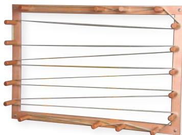
warping frame 11m (37') warp.
